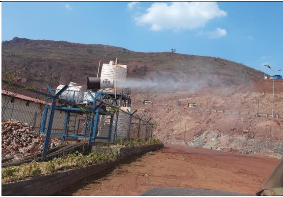
Mist cannon for dust suppression in mineral storage areas
