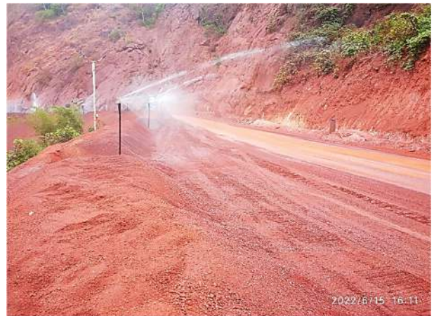
Fixed type sprinkling system on main haul roads for dust suppression
